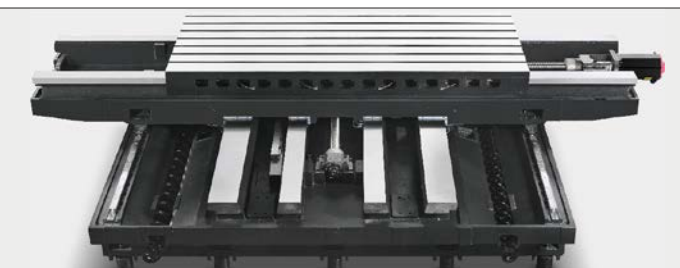
CPV-2200B table base design is with 4 boxway type guideways and 2 linear guideways.
