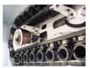
PV series comes with standard 32-tool #50-Chain Type ATC. Dual arm system ensures the stability during tool change. Max. Tool Dia.: 125 mm Tool Length: 350 mm Tool Weight: 20 kgs
